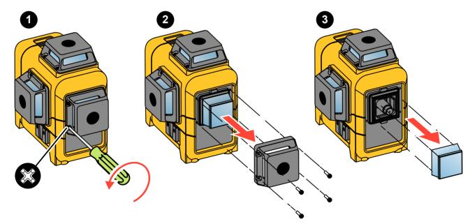
Figure 4. Housing Glass Insert Replacement
