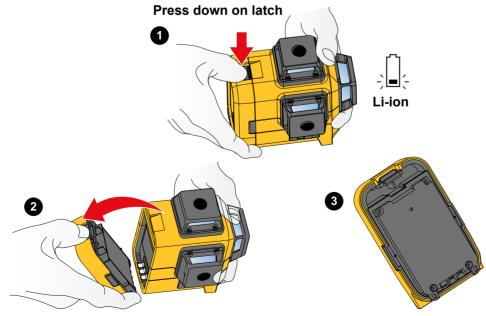
Figure 2. Battery Replacement
