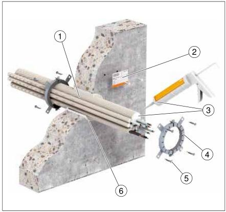
Figure 1: System components
