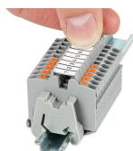
Snapping a marking strip (2009-110) into a marker slot.
