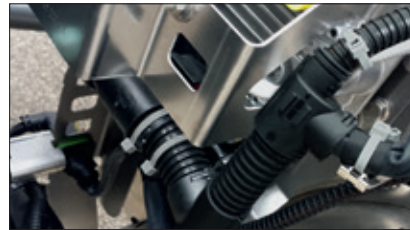
Application of PA46 cable ties at a truck exhaust unit.
