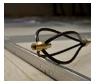
The whisk allows the rod to glide over obstructions easily.
