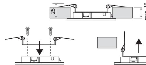
Press leg springs upwards. Insert luminaire into installation opening.
