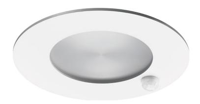
Insaver HE Topper is a ceiling recessed LED downlight with integrated PIR sensor with time (up to 8 mins) and daylight lux level settings. Die-cast aluminium body, Non dimmable LED driver, 8W, 740lm, 93lm/W, 3000K, shallow recessed depth of 55mm.
