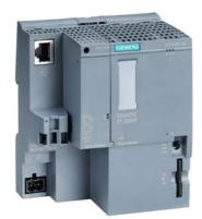
SIMATIC DP, CPU 1512SP-1 PN for ET 200SP, Central processing unit with Work memory 200 KB for program and 1 MB for data, 1st interface: PROFINET IRT with 3-port switch, 48 ns bit performance, SIMATIC Memory Card required, BusAdapter required for Port 1 and 2
