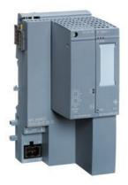
SIPLUS ET 200SP BA 2xRJ45 TX rail based on 6ES7193-6AR00-0AA0 with conformal coating, -40...+70 °C, OT4 with ST1/2 (+85 °C for 10 minutes), BusAdapter 2x RJ45 sockets for PROFINET
