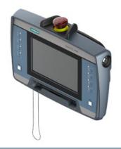
SIMATIC HMI KTP700F Mobile Arctic, (extended operating temperature range), 7.0" TFT display, 800x 480 pixel, 16m colors, key and touch operation, 8 function keys, 1x PROFINET/Industrial Ethernet interface, 1x multimedia card, 1x USB, 1x touch pen, keyswitch, acknowledgement button, emergency shutdown/stop button, configurable from WinCC Comfort V15 SP1
