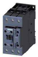
power contactor, AC-3 40 A, 18.5 kW / 400 V 1 NO + 1 NC, 24 V AC 50 Hz, 3-pole, Size S2, screw terminal upright mounting position
