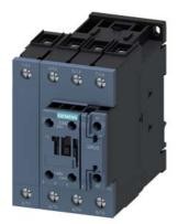
Contactor, AC-1, 60 A/400 V/40 °C, S2, 4-pole, 230 V AC/50 Hz, 1 NO+1 NC, screw terminal
