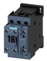
Power contactor, AC-3 38 A, 18.5 kW / 400 V 1 NO + 1 NC, 220 V AC 50 Hz, 240 V, 60 Hz 3-pole, Size S0, screw terminals
