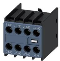
auxiliary switch, on the front, 1 NO + 3 NC, .1/.2, .1/.2, .1/.2, .3/.4, current path: 1 NC, 1 NC, 1 NC, 1 NO, screw terminal, for contactors 3RT2 and contactor relays 3RH2
