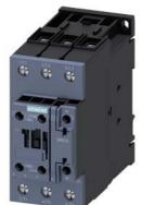
power contactor, AC-3 51 A, 22 kW / 400 V 1 NO + 1 NC, 230 V AC 50 / 60 Hz, 3-pole, size S2, screw terminal
