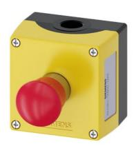
Enclosure for command devices, 22 mm, round, Enclosure material metal, Enclosure top part yellow, 1 control point metal, A=EMERGENCY STOP mushroom pushbutton red, 40 mm, rotate-to-unlatch, Control point in center, 2 NC, screw terminal, floor mounting, 1xM20 each on top and bottom
