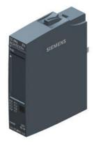
SIPLUS ET 200SP DQ 8x24VDC/0.5A HF based on 6ES7132-6BF00-0CA0 with conformal coating, -40...+70  $^{\circ}$ C, digital output module, suitable for BU type A0, color code CC02, channel diagnostics,
