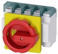
SENTRON, Switch disconnector 3LD, emergency switching-off switch, 4- pole, 100 A, operating power at AC-23 A at 400 V: 37 kW, front-mounted, rotary operating mechanism, Red / yellow, 4-hole mounting of the handle
