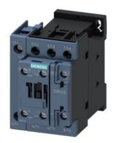
contactor AC-1, 35 A, 400 V / 40 °C, 4-pole, 230 V AC, 50 Hz, auxiliary contacts: 1 NO + 1 NC, screw terminal, size: S0
