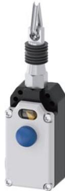
cable-operated switch metal enclosure, 2 xM20 x1.5; 1 NO+1 NC, latching, ISO 13850 and button reset, for wire lengths up to 20 m
