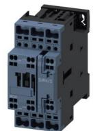
power contactor, AC-3e/AC-3, 38 A, 18.5 kW / 400 V, 3-pole, 24 V AC, 50/60 Hz, auxiliary contacts: 1 NO + 1 NC, spring-loaded terminal, size: S0
