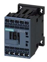
power contactor, AC-3e/AC-3, 9 A, 4 kW / 400 V, 3-pole, 220 V AC, 50/60 Hz, auxiliary contacts: 1 NC, spring-loaded terminal, size: S00  $\,$
