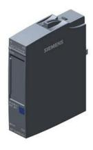
SIPLUS ET 200SP AI 2xU/I 2-, 4-wire HS based on 6ES7134-6HB00-0DA1 with conformal coating, -40...+60  $^{\circ}$ C, analog input module, suitable for BU type A0, A1, color code CC00, channel diagnostics, 16-bit, +/-0.3%
