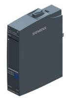
SIPLUS ET 200SP AI 4xU/I 2-wire T1 rail based on 6ES7134-6HD01-0BA1 with conformal coating, -40...+60 °C, OT1 with ST1/2 (+70 °C für 10 minutes), analog input module, suitable for BU type A0, A1, color code CC03, module diagnostics, 16 bit, +/-0.3%
