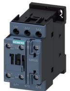
power contactor, AC-3e/AC-3, 25 A, 11 kW / 400 V, 3-pole, 230 V AC, 50/60 Hz, auxiliary contacts: 1 NO + 1 NC, screw terminal, size: S0
