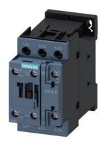
power contactor, AC-3e/AC-3, 17 A, 7.5 kW / 400 V, 3-pole, 230 V AC, 50/60 Hz, auxiliary contacts: 1 NO + 1 NC, screw terminal, size: S0
