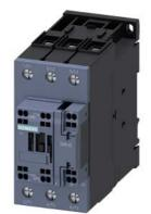
power contactor, AC-3e/AC-3, 41 A, 18.5 kW / 400 V, 3-pole, 230 V AC, 50/60 Hz, auxiliary contacts: 1 NO + 1 NC, main circuit: screw terminal, control and auxiliary circuit: spring-loaded terminal, size: S2
