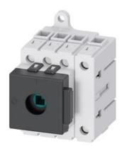
Load disconnector 3LD3, Iu 63 A Main switch 3-pole + N Rated operating capacity at AC-23 A at 400V 22.0 kW Installation in distribution boards, Basic switch without Knob-operated mechanism
