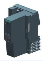
SIPLUS ET 200SP IM155-6PN ST based on 6ES7155-6AU01-0BN0 with conformal coating, -40...+70 °C, PROFINET interface module, 1 slot for BusAdapter, max. 32 I/O modules, and 16 ET 200AL modules, single hot swap, including server module (6AG1193-6PA00-7AA0)
