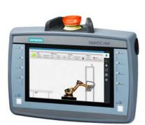
SIMATIC HMI KTP700F Mobile, 7.0" TFT display, 800x 480 pixel, 16m colors, key and touch operation, 8 function keys, 1x PROFINET/Industrial Ethernet interface, 1x multimedia card, 1x USB, Key-operated switch, acknowledgement button, 1 emergency stop/stop button configurable from WinCC Comfort V13 SP1
