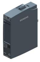
SIPLUS ET 200SP DQ 8x24V DC/0.5A Sink Basic based on 6ES7132-6BF61-0AA0 with conformal coating, -40...+70  $^{\circ}$ C, digital output module, suitable for BU type A0, color code CC01
