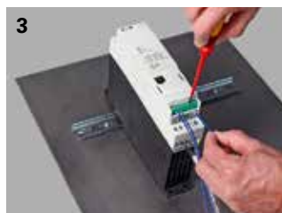
3 Connect the control current.
