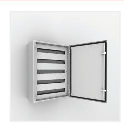
**Omschrijving:** Used for easy mounting of DIN-rail components with a maximum height of 68 mm. Distance between rows 125 mm. If required, the standard enclosure door can be replaced with a glazed door. Usable depth between front cover and external door: 35 mm. In stainless steel enclosure machining is required.
