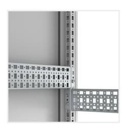
**Omschrijving:** Universal profile for both depth and width fitting on the 25 mm DIN hole pattern of the enclosure's frame or in combination with the CLPF and VB profiles. The 75 mm wide profile is equipped with three rows of holes of which one is turned 90°. This makes it possible to mount the CLPF profiles in both directions. The CLPK can be secured by the use of self tapping screws.
