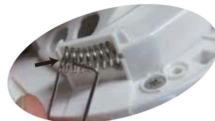
Figure 4, Push the spring to the right side to let it is held by right arm
