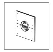
9. Insert the E-BFDC valve into the duct at a depth of 20 mm from the wall surface so that the blade is oriented in the direction of the duct.
