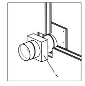
7. Completely fill the S connection between the duct and the wall with rock wool (density of at least  $100 \text{ kg} / \text{m}^3$ )
