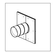
10. Place the fire damper cartridge in the conduit so that the face of the cartridge is 45 mm from the surface of the wall. A E-BFDC must be mounted so that the mouth is positioned against the wall
