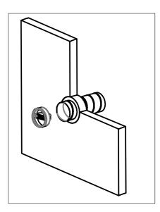
3. Insert the damper into the duct at a depth of 20mm from the wall surface so that the blade is oriented in the direction of the sheath.
