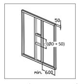
1. Provide an opening of at least  $= (ØD + 50) \text{ mm } \times (ØD + 50) \text{ mm}$
