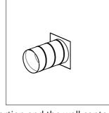
5. Coat the wool filler, the sheath portion and the wall contact points and fill the rock wool with a fire-resistant coating in the thickness of 2 mm.
