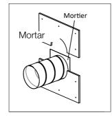
7. Fill the gap between the wall and the valve with plaster, cover it with the GKF plate and tighten it with screws.
