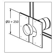
6. Install another layer of GKB plates perpendicular to the first layer and tighten with 5.5x70 mm self-tapping screws.
