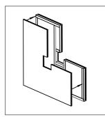
3. Insulate the wall entirely with rockwool (40 mm - 100 kg / m<sup>3</sup>) and finish with two GKF plaster lacquers.
