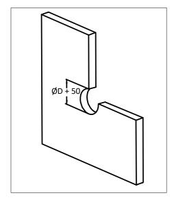
1. Provide an opening in the wall / slab / ceiling of at least =  $\emptyset D + 50$  mm.
