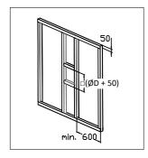
1. Provide an opening of at least  $= (ØD + 50) \text{ mm} \times (ØD + 50) \text{ mm}$ + horizontal consolidations in the wall
