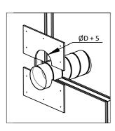
5. Cover with another GKF plate of the same dimensions and tighten with self-tapping 5.5x70 mm screws.
