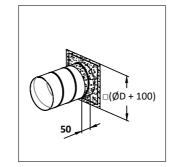
6. Insert the E-BFDC valve into the duct at a depth of 20 mm from the wall surface so that the blade is facing in the direction of the duct.
