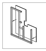
2. Attach two GKF plasterboards 12.5 mm thick to one side of the stud wall. For a metal stud wall with 90 ' fire resistance, use fire-resistant plasterboard of the same thickness.
