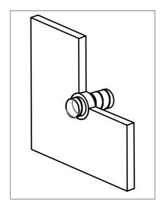
2. Place a metal conduit in the opening. The clearance between the duct and the wall / slab / ceiling must be filled completely with mortar
