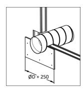
4. Insert the ventilation duct into a hole in the wall and press it on the GKF plate of width (ØD + 250mm) and with the central hole (ØD + 5mm), then tighten with self-tightening screws. tapping machines 5,5x70 mm.
