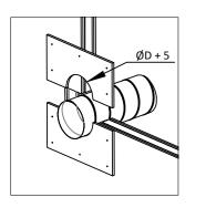
5. Cover with another GKB plate of the same dimensions and tighten with self-tapping screws 5.5x70 mm.
