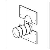
8. Complete the filling with a layer of GKB plates and tighten them with the 5.5x70 mm screws.
