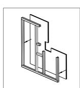
2. Attach two GKB plasterboards 12.5 mm thick to one side of the stud wall. For a metal stud wall with 60 'fire resistance, use fire-resistant plasterboard of the same thickness.
