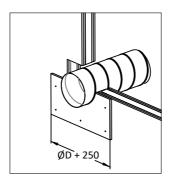
4. Insert the ventilation duct into a hole in the wall and press it on the GKB plate of width (ØD + 250mm) and with the central hole (ØD + 5mm), then tighten with self-tightening screws. tapping machines 5,5x70 mm.
