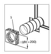
4. Insert the ventilation duct into a hole in the wall and fill the gap between the duct and the wall with two layers of mineral wool 100 kg / m<sup>3</sup> density, 50 mm thick and (ØD + 200) mm width . The outer and inner edges as well as the tactile surfaces between the layers of wool should be previously primed fireproof coating.
