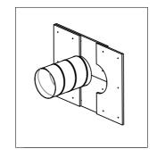
8. Install another layer of GKF plates perpendicular to the previous one and tighten with screws.
