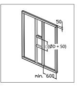
1. Provide an opening of at least  $= (ØD + 50) \text{ mm } \times (ØD + 50) \text{ mm}$
