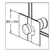
6. Install another layer of GKF plates perpendicular to the first layer and tighten with self-tapping 5.5x70 mm screws.
